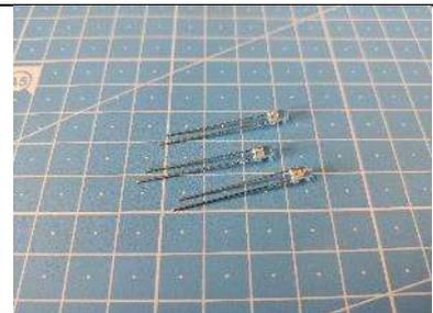
3x Phototransistor PT204-6C
